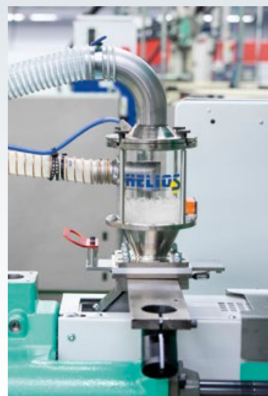
HELIOS®Clean 2 on processing machine Control version CE as second conveying point of JETBOXX® dryer
