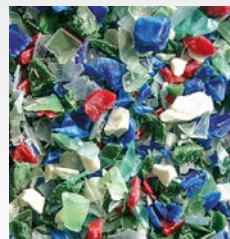
grinding material from shredder
