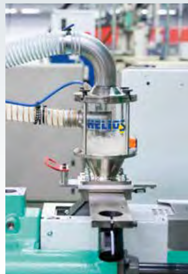
HELIO® Clean 2 on processing machine Control version CE as second conveying point of JETBOXX® dryer
